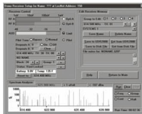
The lower section of the display provides a graphical, scanning spectrum analyzer for conducting site surveys. During scanning, the receiver is tuned in steps across its tuning range and markers are placed on the screen to indicate the frequency and signal strength of signals found.
