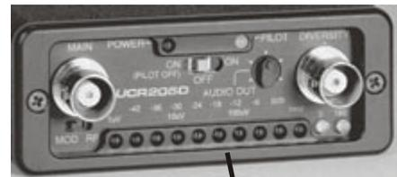
Receiver front panel LED strip for monitoring.
