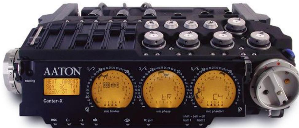
AATON CANTAR-X is an 8-track sound recorder with a hard disk, designed for recording sound on location. The equipment has an integrated mixing console with 18 inputs (5 mics, 4 line analogue and 8 digital inputs) and digital recording on a hard drive.
