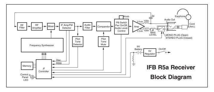
The incoming RF signal is filtered and amplified, then mixed down to the IF frequency with a microprocessor controlled synthesizer. The pilot tone signal is on a different frequency than Lectrosonics wireless microphone systems to prevent interference when the wireless microphone and IFB systems are used in the same location. The audio signal processing includes compandor noise reduction for low noise and excellent intelligibility.
